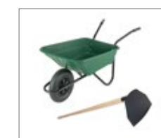
Wheelbarrow / Hoe (mortar preparation)
