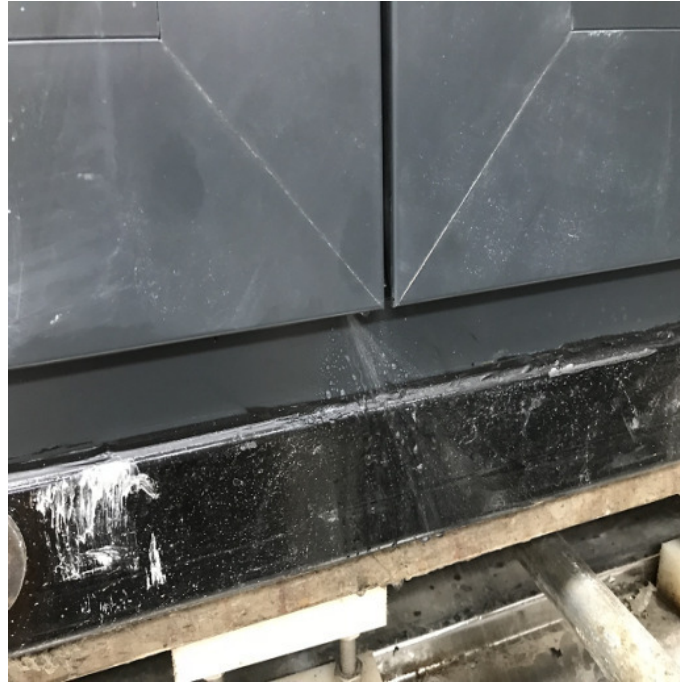
Photo 4. A view of water leakage (Test No: 2018.963.01 / 16.02.2018)
